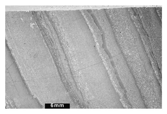
Figure 4.19. Person County sample with sedimentary laminae, grading (top to the right), and micro-faults (FBL046; scanned thin section, plane-polarized light).
