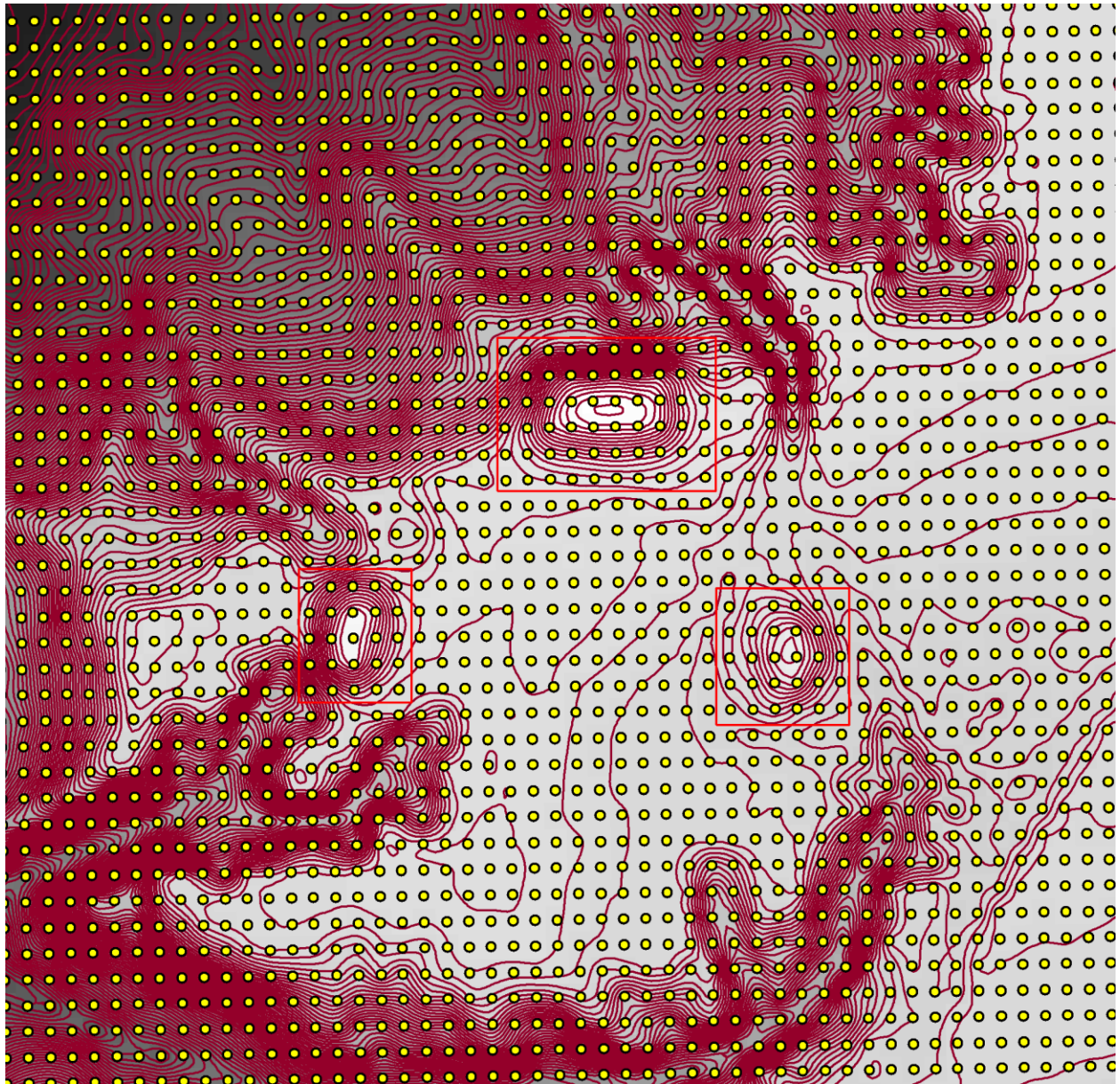
3 rd Arc-Second LiDAR Coverage (approx. 10 m spacing of data points). ArcGIS map view.
