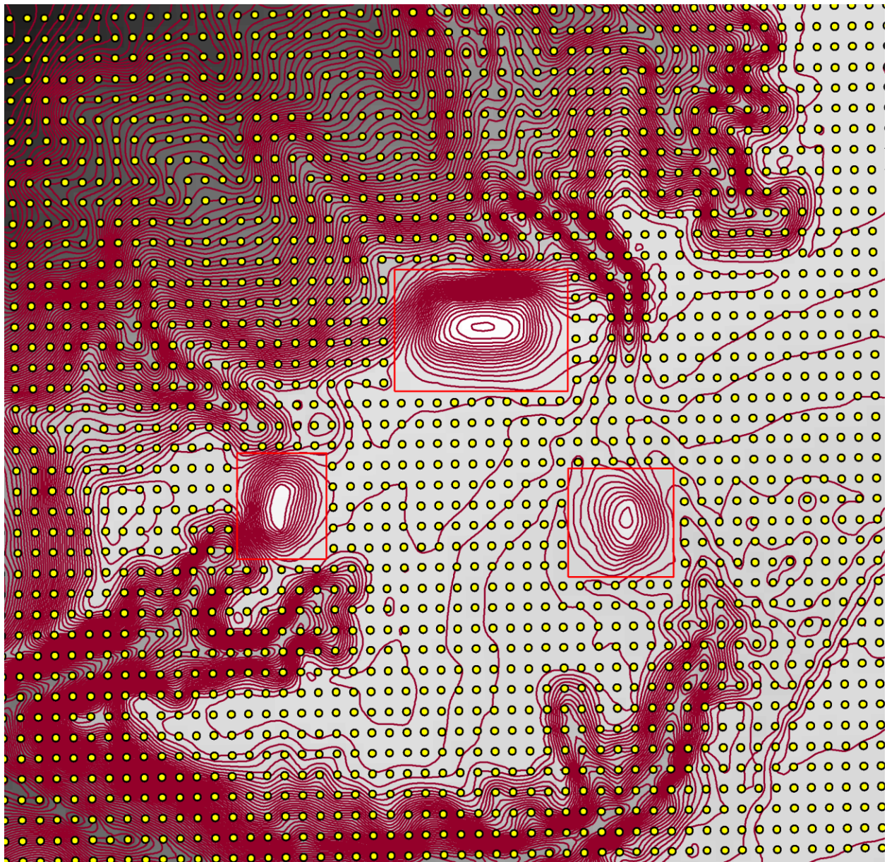
3 rd Arc-Second LiDAR Coverage with points removed from mounds. ArcGIS map view.
