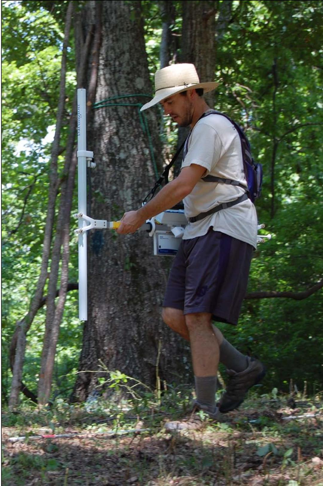
Figure 3. Edward Henry collecting gradiometer data with a single-sensor Bartington Instruments, Inc. Grad-601-2. Photograph by David Cranford.
