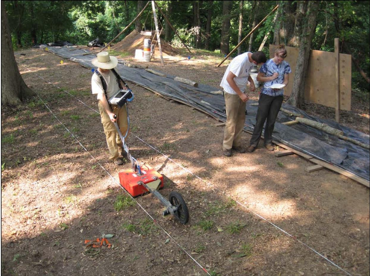
Figure 4. GPR data being collected atop Mound B with the GSSI SIR-3000 and 270 MHz antenna. Alex Craib and Sara Wyatt taking positional notes. Photograph by Vin Steponaitis.
