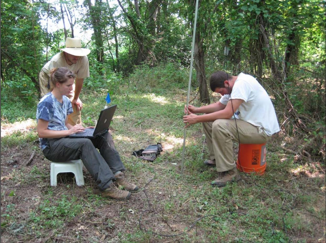
Figure 6. Down-hole data collection underway with the Bartington Instruments, Inc. MS2H sensor, MS2 meter, and field laptop. Photograph by Vin Steponaitis.
