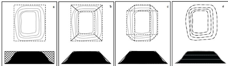
Figure 2: (a-c) Geometric methods of calculating volume, all leading to significant over-estimation; (d) the more accurate contour method of calculating volume (Lacquement 2009:Figures 2.1-2.2).
