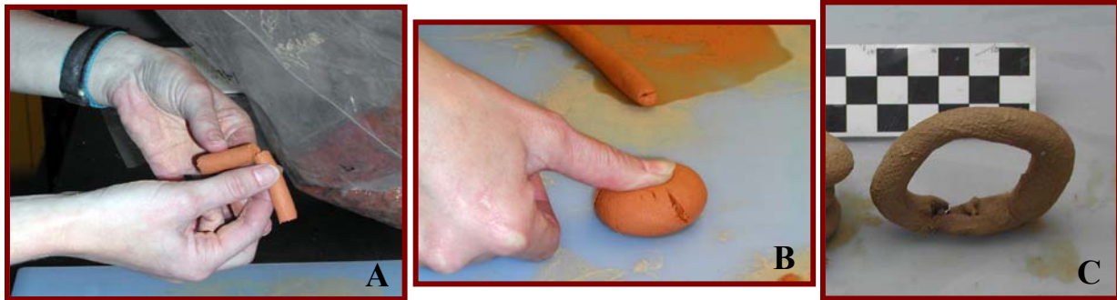
Figure 4. The plasticity and stiffness of each sample was judged in the lab on the basis of coil (A), ball (B), and loop (C) tests.
