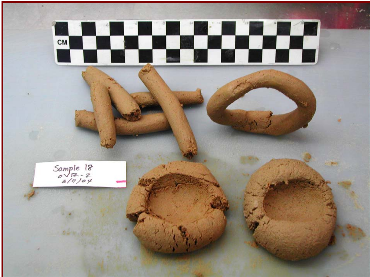
Figure 5. In general, lean clays are defined as those having coils that break completely when wrapped, rings that sag significantly when stood on edge, and balls that develop deep cracks when compressed.
