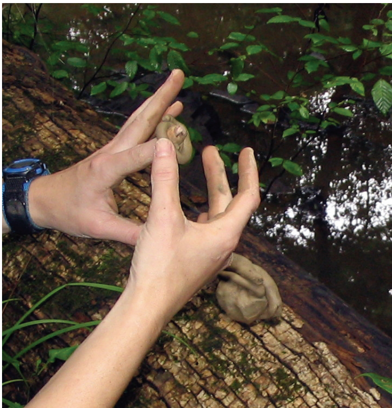
Figure 4.1. “Coil” test to evaluate plasticity.
