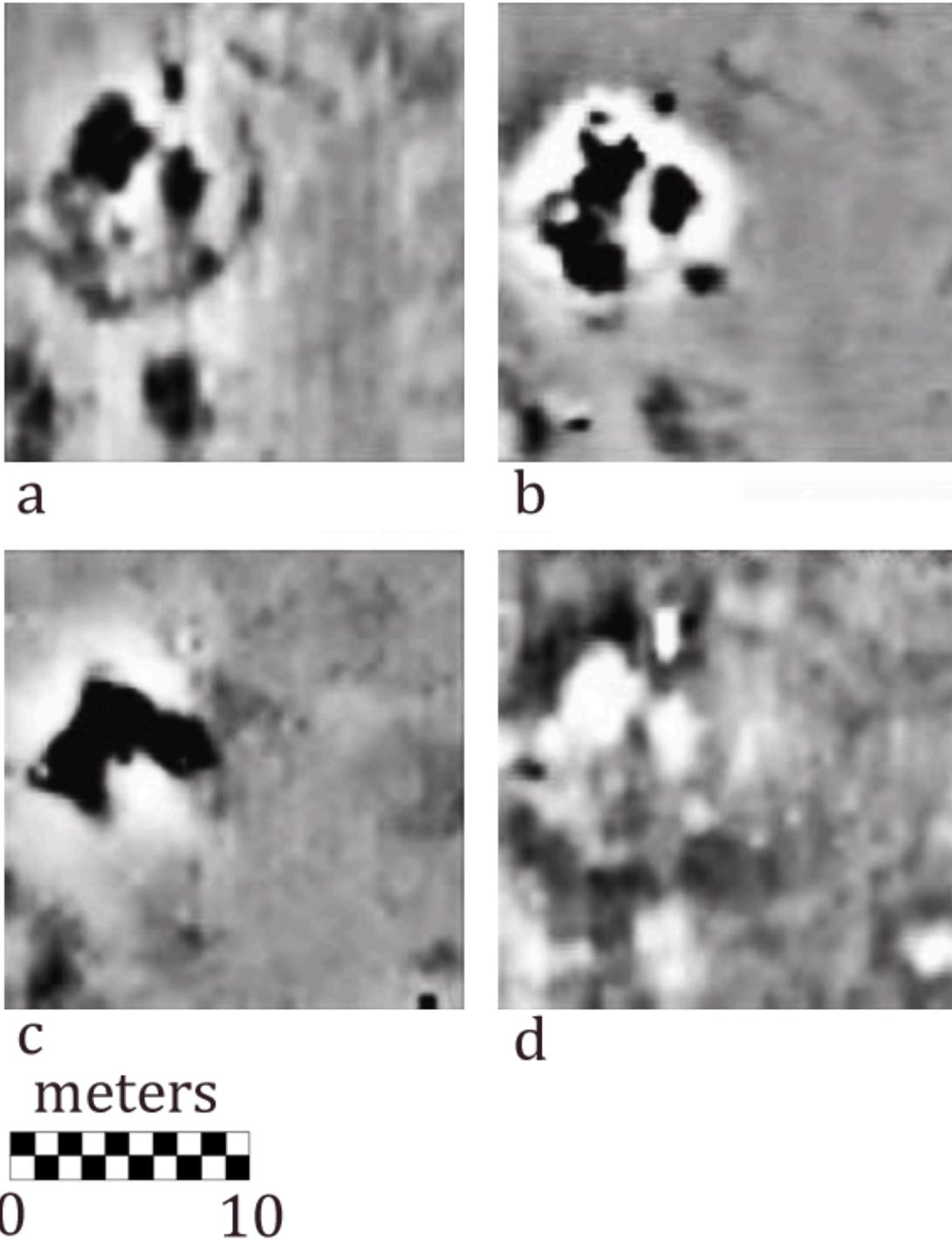
Figure 4.1. Complementary geophysical surveys of a 15th century Caddo structure at a site in southwest Arkansas: 1) magnetic susceptibility; b) magnetometry; c) electrical resistance; d) electromagnetic conductivity (adapted from Lockhart and Green 2006:Figure 2.8)
