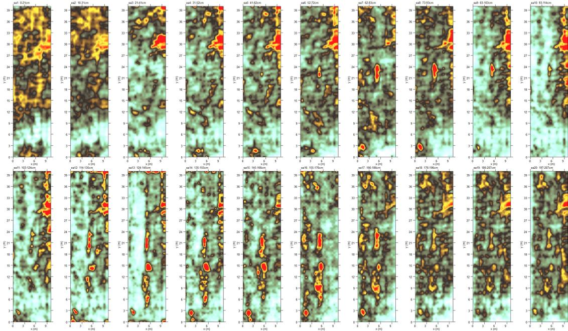
Figure 4.7. The original 20 GPR slices, later interpolated into 77 slices. The cultural zone is likely represented in the first 10 slices whereas the subsoil zones are captured in the next 10 slices.
