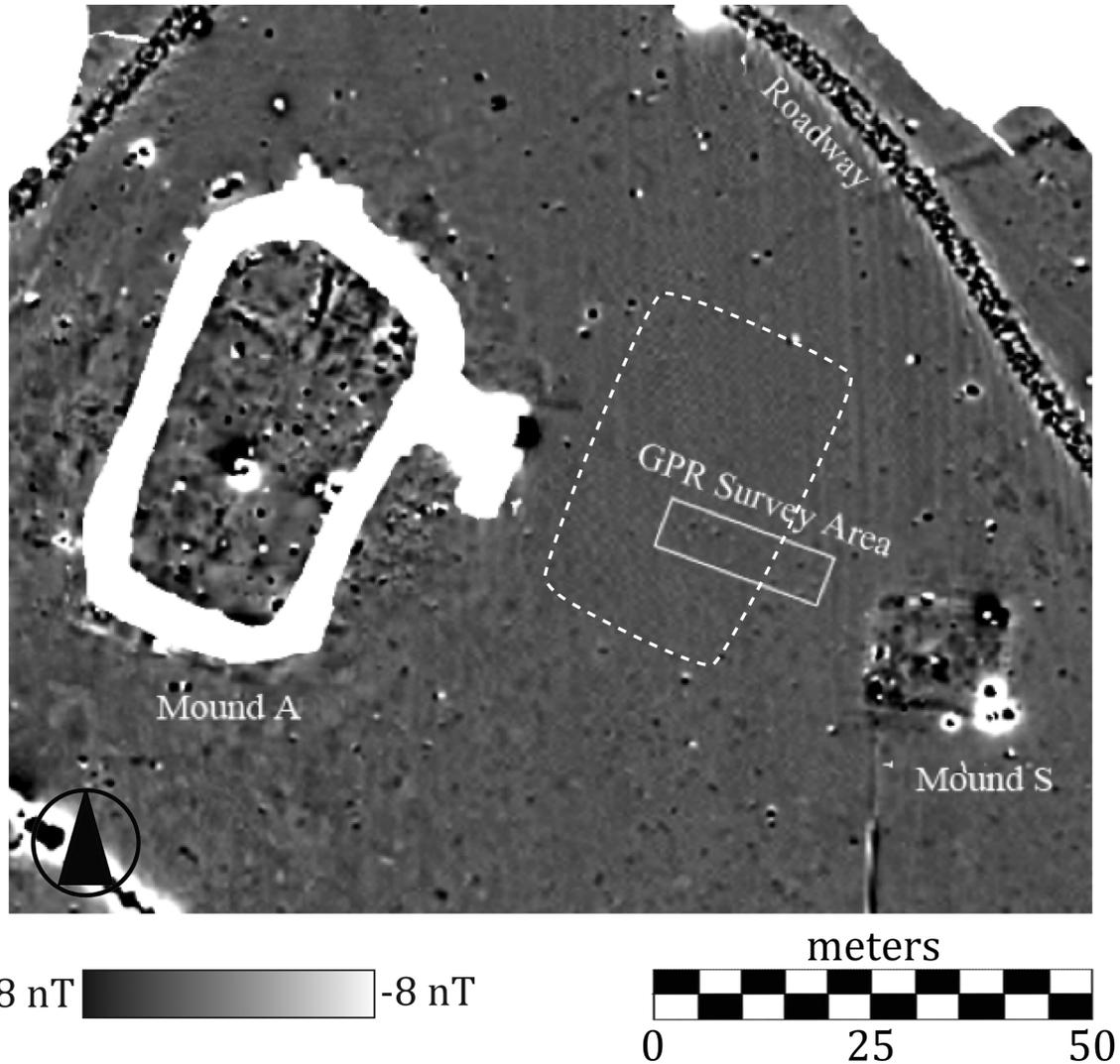
Figure 4.6. Section of the 2010 magnetometer survey area including mounds A and S. The possible architecturally delineated plaza, inside the broken line, lies between the two mounds and is the approximate size and orientation of Mound A. The GPR collection area, inside the solid line, was positioned so as to overlap this feature of the landscape and the band of supposed architecture surrounding it.
