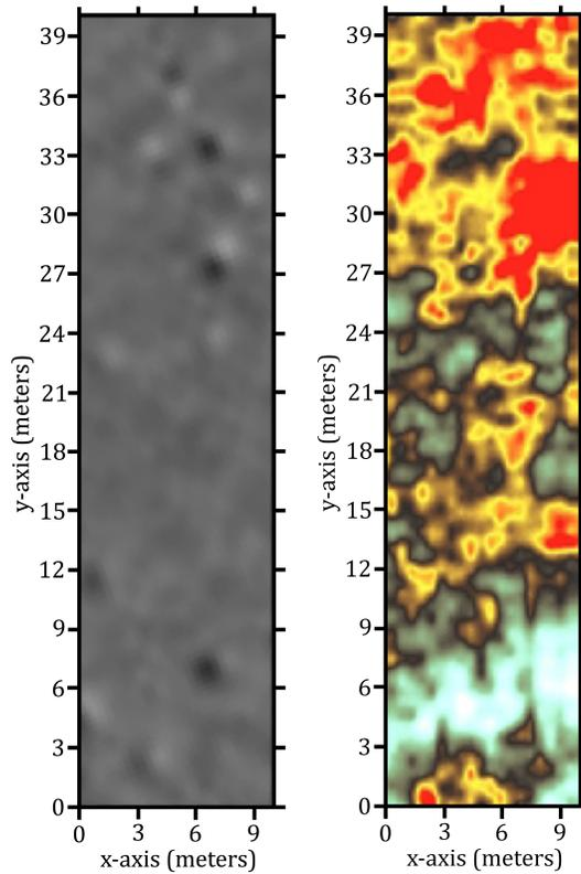
Figure 4.8. Magnetometer (left) and GPR (right) data for the 10-x-40 meter collection area. East end of survey area is at the bottom of the image.
