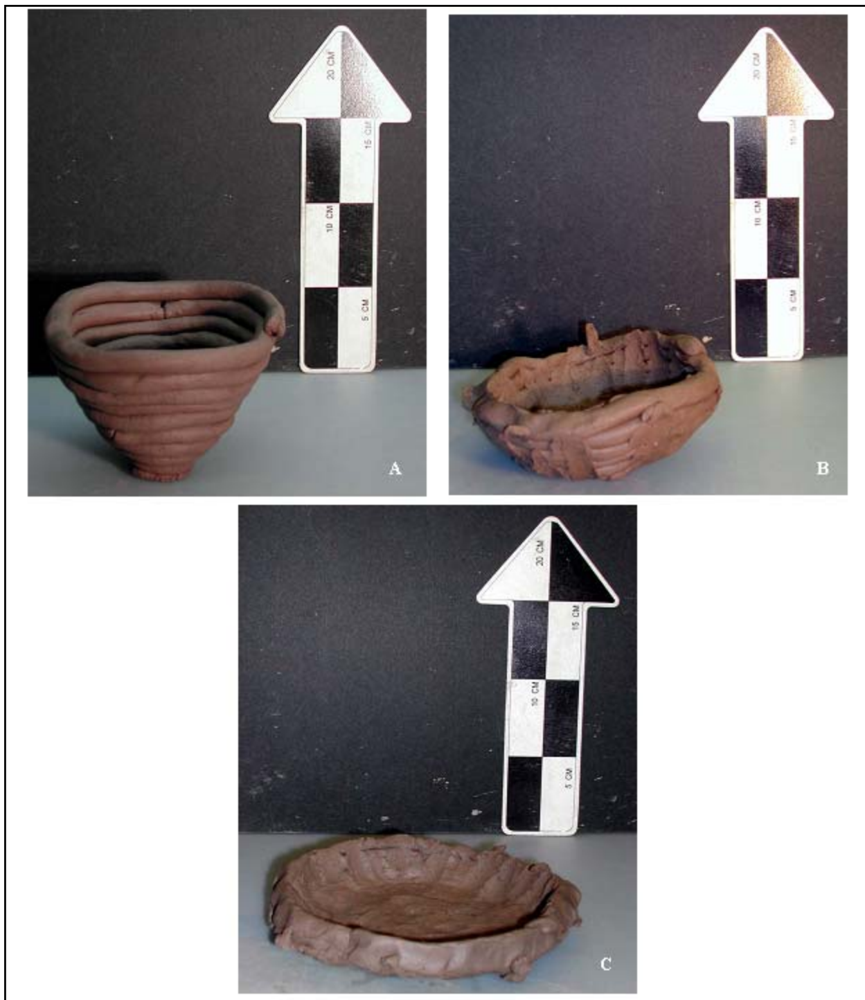
Figure 12. Process of building a vessel from a “fat” clay collected in an alluvial setting: (A) addition of coils to build up vessel walls, (B) smoothing of vessel walls accompanied by noticeable slumping, and (C) complete collapse of vessel under its own weight.
