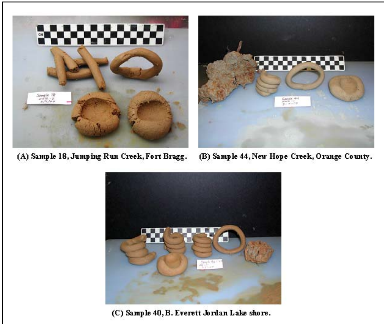
Figure 7. Clays exhibiting varying degrees of plasticity: (A) lean clay; note that the coil has broken into short segments, the ring is sagging and twisting, and the ball has developed deep cracks; (B) moderately lean clay; note that the coil has cracked, the ring is sagging slightly, and the ball has developed shallow cracks; and (C) good clay; note that the coils have not cracked, the ring does not sag, and the ball has not cracked.
