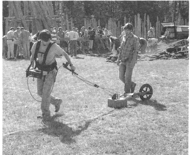
Jonathan Flood pulls a GPR (ground penetrating radar) unit over the site surface at Town Creek to detect buried features.
